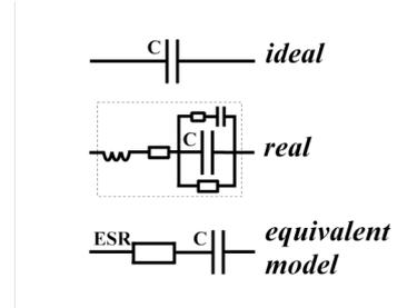
**Fig. 1. Ideal capacitor. Real capacitor [3] with additional parasitic components (inductive element is not significant on SMD capacitor technology for our frequency range). Equivalent model with Equivalent Series Resistance (ESR).**
