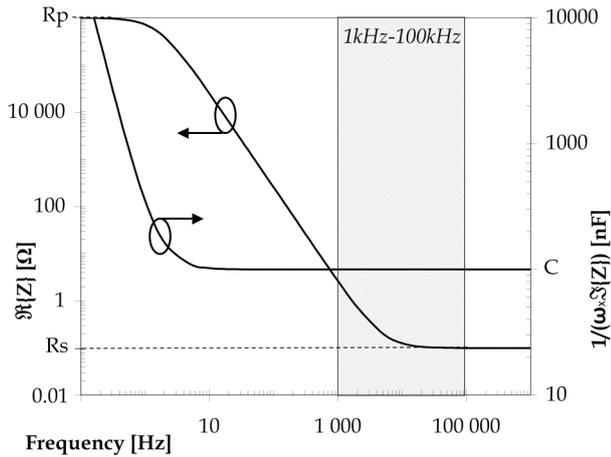
**Fig. 5. Evolution of the ESR (5) and Capacitance (6) following a first approximation parasitic model of capacitor given on figure 4 (numerical application:  $C = 100$  nF,  $R_p = 1$  MΩ and  $R_s = 0.1$  Ω).**
