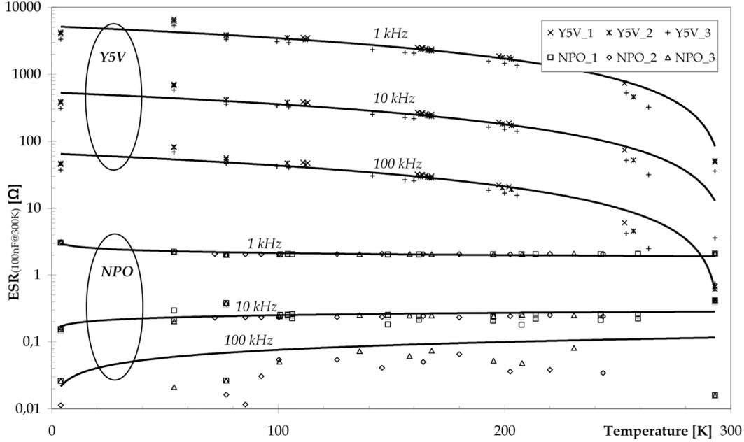
**Fig. 3.** NPO and Y5V equivalent series resistance (ESR) normalized for 100 nF capacitance at 300 K as a function of temperature. Measurement was made at intermediate temperatures in the cold helium gas.
