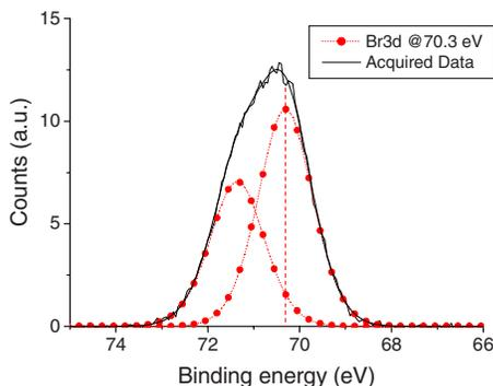
FIG. 8. (Color online) Br  $3d$  core level spectrum of thin (2.5 nm)  $\text{SiO}_2$  layer measured by XPS at  $23.75^\circ$  after exposure to  $\text{HBr}/\text{O}_2/\text{Ar}$  plasma pulsed at 5 kHz and 20%.
