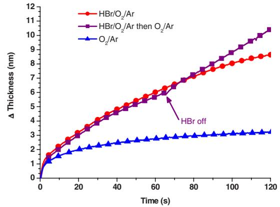
FIG. 12. (Color online) Damaged thickness measured by kinetic *in situ* ellipsometry as a function of plasma exposure time in cw mode during a  $\text{HBr}/\text{O}_2/\text{Ar}$  or a  $\text{O}_2/\text{Ar}$  plasma and a  $\text{HBr}/\text{O}_2/\text{Ar}$  plasma followed by  $\text{O}_2/\text{Ar}$  plasma.
