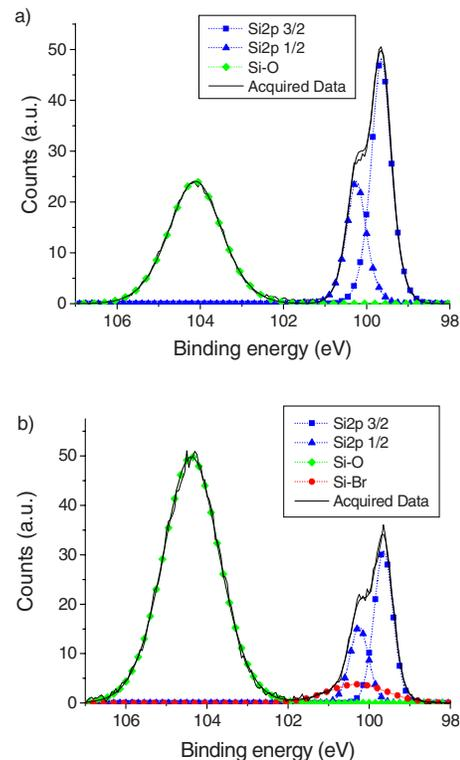
FIG. 3. (Color online) Si  $2p$  core level spectra of thin (2.5 nm)  $\text{SiO}_2$  layer measured by XPS at  $23.75^\circ$  (a) before and (b) after exposure to  $\text{HBr}/\text{O}_2/\text{Ar}$  plasma in cw mode.
