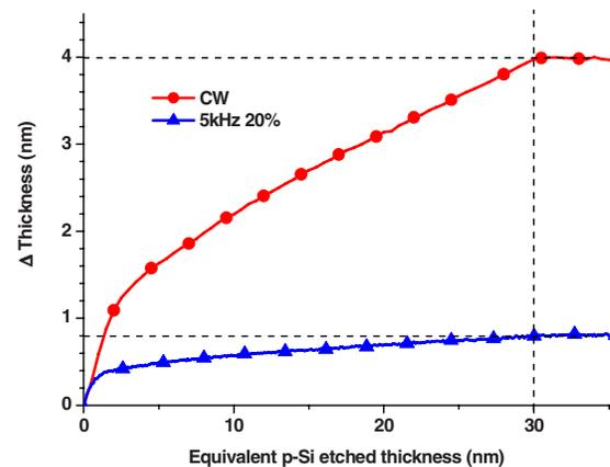
FIG. 6. (Color online) Damaged thickness measured by kinetic *in situ* ellipsometry as a function of equivalent poly-Si etched thickness in cw mode and synchronous pulsing mode with 5 kHz and 20% of duty cycle.
