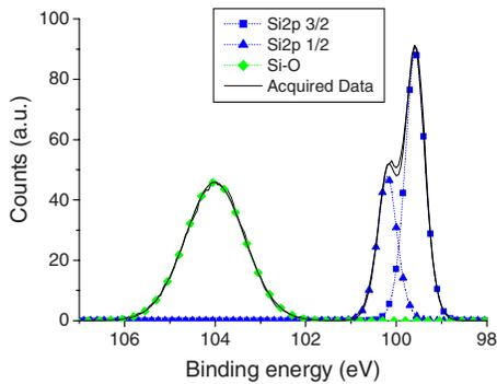
FIG. 7. (Color online) Si  $2p$  core level spectrum of thin (2.5 nm)  $\text{SiO}_2$  layer measured by XPS at  $23.75^\circ$  after exposure to  $\text{HBr}/\text{O}_2/\text{Ar}$  plasma pulsed at 5 kHz and 20%.
