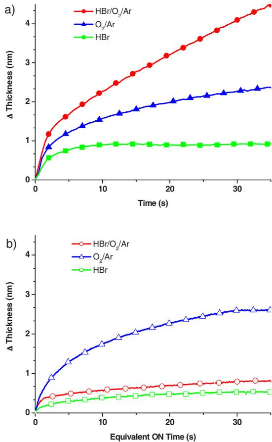
FIG. 10. (Color online) Damaged thickness measured by kinetic *in situ* ellipsometry as a function of plasma exposure time in (a) cw mode and (b) synchronous pulsing mode with 5 kHz and 20% of duty cycle for HBr/O<sub>2</sub>/Ar, O<sub>2</sub>/Ar, and HBr plasma.
