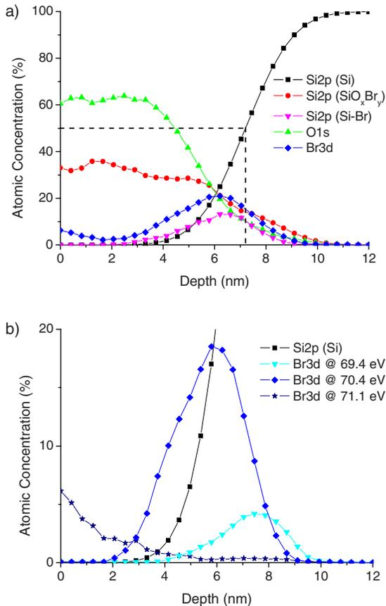
FIG. 5. (Color online) Atomic concentration depth profile of  $\text{SiO}_2$  layer exposed to  $\text{HBr}/\text{O}_2/\text{Ar}$  plasma in cw mode: (a) global depth profile and (b) decomposition of Br profile.
