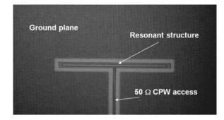
Fig. 13. Folded-slot antenna on a HR silicon substrate.
