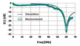
Fig. 14. Folded-slot antenna matching.
