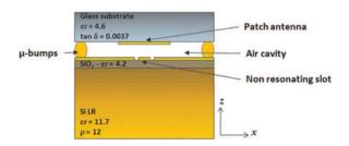
Fig. 18. Side view of the Si-IPD  $^{\text{TM}}$  packaged antenna.
