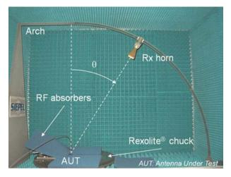
Fig. 1. STMicroelectronics measurement setup for gain characterization.
