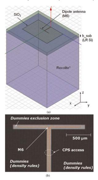
Fig. 7. Dipole antenna integrated on a LR substrate (a) model, and (b) microphotograph of the integrated antenna.
