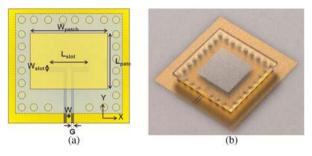
**Fig. 19.** Top view of the Si-IPD<sup>TM</sup> packaged antenna (a) and photo of a patch antenna on  $IPD^{TM}$  mounting (b).
