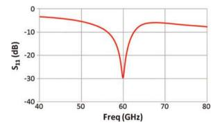
Fig. 20. Simulated return loss of the Si-IPD antenna.
