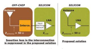
Fig. 4. Co-integration technique in an SoC approach.
