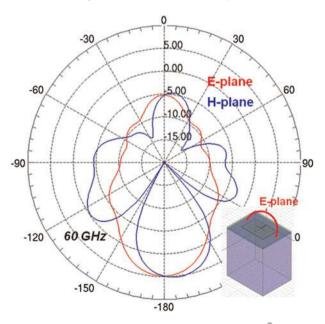
Fig. 9. Simulated radiation pattern of the standalone antenna at 60 GHz.
