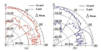
Fig. 12. Measured and simulated radiation pattern of the dipole antenna on 235  $\mu$ m-height substrate: (a) *E*-plane and (b) *H*-plane.
