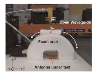
Fig. 3. Lab-STICC measurement setup for radiation pattern characterization.
