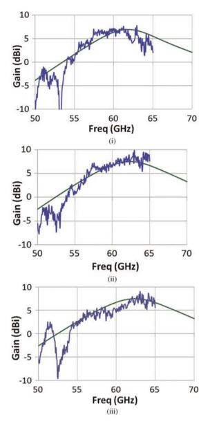
Fig. 25. Measured and simulated gain versus frequency for three cavity heights:  $h = 75 \ \mu m$  (i);  $h = 125 \ \mu m$  (ii); and  $h = 250 \ \mu m$  (iii).
