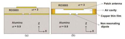
Fig. 23. Side view of the different packaged Alumina-RO3003 antenna configurations: without (a) and with intermediate air cavity (b).
