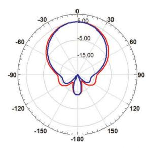
Fig. 21. Simulated radiations patterns at 60 GHz: *E* (blue) and *H* (red) planes.
