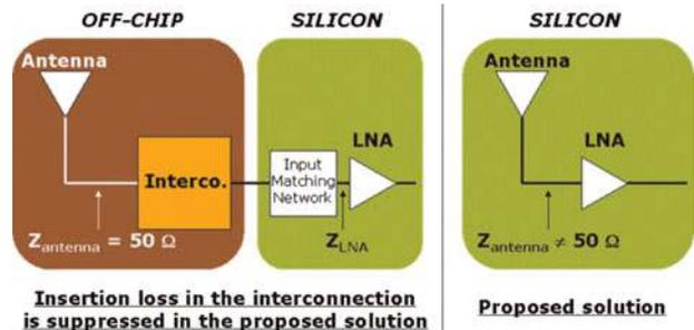
Fig. 4. Co-integration technique in an SoC approach.
