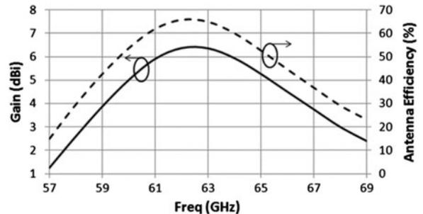
Fig. 22. Simulated gain and antenna efficiency versus frequency in  $z > 0$  (LR Si).
