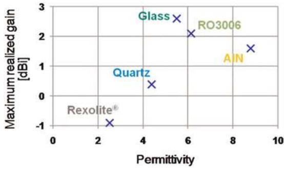
Fig. 16. Maximum realized gain versus “lens” material permittivity with 3 mm height.
