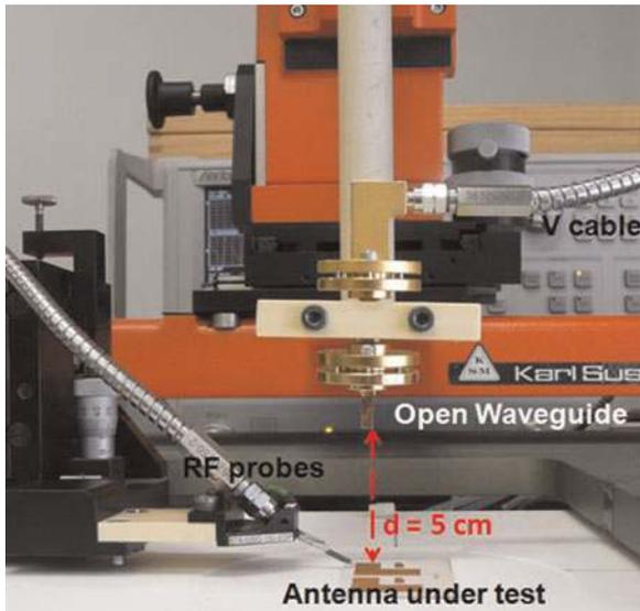
Fig. 2. Lab-STICC measurement setup for gain characterization.
