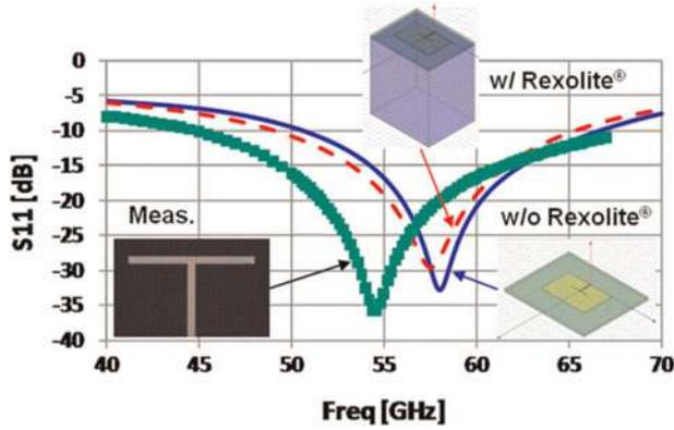
Fig. 8. Comparison of  $S_{11}$  for two configurations (w/ and w/o Rexolite<sup>®</sup>) and measurement.
