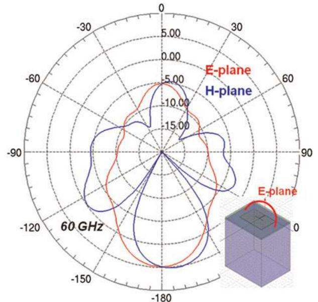
Fig. 11. Simulated radiation pattern of the antenna with Rexolite<sup>®</sup> at 60 GHz.
