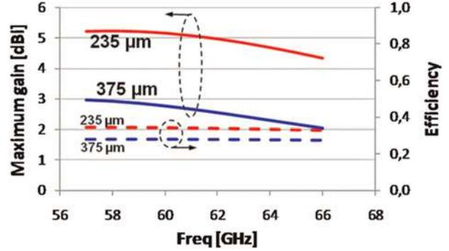
Fig. 10. Maximum gain and efficiency versus frequency.
