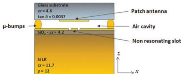
Fig. 18. Side view of the Si-IPD™ packaged antenna.
