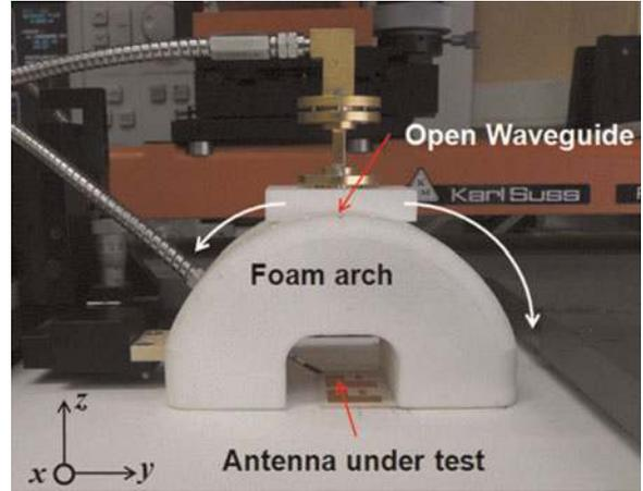
Fig. 3. Lab-STICC measurement setup for radiation pattern characterization.
