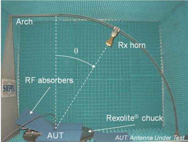
Fig. 1. STMicroelectronics measurement setup for gain characterization.
