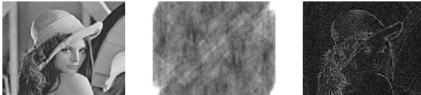
Fig. 1.1. The Phase only inverse Vs. Magnitude Only inverse - left: original, middle: magnitude only, right: phase only
