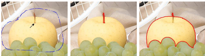
Fig. 12. Example comparison of Graph cuts and Power watershed faced to a weak foreground seeds quantity. (a) Seeds (the foreground seed is in red, indicated by an arrow), (b) Graph cuts segmentation result, (c) Power watershed ( q = 2 ) result.
