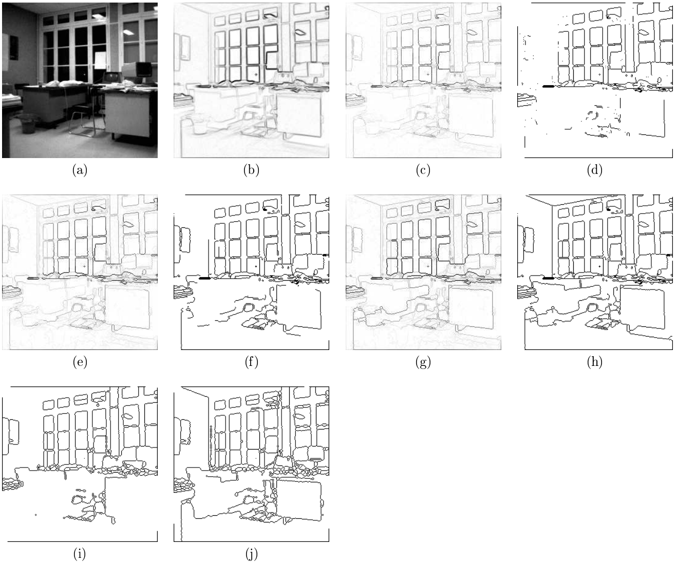
Figure 13. Crest restoration. (a): original image; (b): after Deriche gradient operator (the lowest values appear in white); (c): after a filtered thinning; (e): after 10 steps of CrestRestoration; (g): after iterating CrestRestoration until stability; (d,f,h): threshold at the same level of (c,e,g) resp.; (i,j): hysteresis thresholding.
