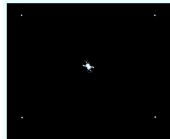
Fig. 5 : Fourier transform showing Bayer interpolation peaks.
