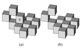
Figure 1. A lump, made of 11 voxels, is depicted in (a). It contains no simple voxel, and is simple-equivalent to the complex in (b), made of 10 voxels. Both objects have three tunnels.
