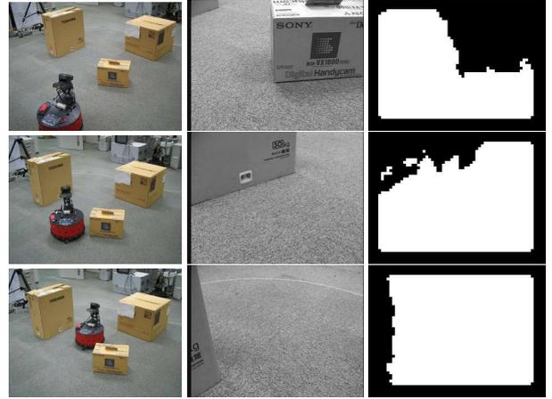
Figure 17: The left column shows the images of the experimental environment, the middle column shows the images observed by the mobile robot, and the right column shows the dominant planes computed by our algorithm. The top, middle, and bottom rows are captured at frame 16, 68, and 100, respectively.
