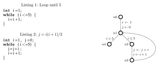
This example is not fortuitous: it models how to address consecutive lines of a matrix in lower triangular packed storage mode. In that memory-effective approach, the matrix is stored in memory as a unidimensional array, each line next to the preceding one, and line number i only uses i positions in the array: j is the index of the start of the line in the array.
