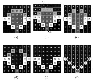
**Fig. 2.** (a): Original image. (b-f): several steps of the flooding algorithm. One can see that this algorithm is not "monotone": some points at altitude 10 are processed after one of the points at altitude 20. One can also note that the contour at altitude 20 in the original image (a) is not present in the result (f).
