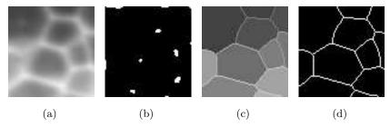
**Fig. 1.** (a): original image, (b): regional minima of (a) (in white), (c): a topological watershed of (a), (d): a divide set of (a), obtained by taking the complement of the regional minima of (c).
