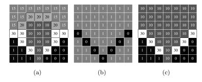
**Fig. 5.** (a) An image F, and (b) the flooding extension of F, and (c) the associated mosaic.
