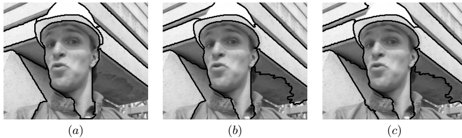
Fig. 5. Results (superimposed in black to the original image), obtained by applying a watershed on (a) an edge-weighted graph and (b, c) a vertex-weighted graph. In (a), a filtered version of the function derived from the image as described in Sec. 1 is considered. In (b) (resp. (c)) a filtered version of the Deriche edge detector (resp. morphological gradient) is considered. In each case, a filtering step, based on area closing [15], ensures that the watershed defines exactly 12 catchment basins.
