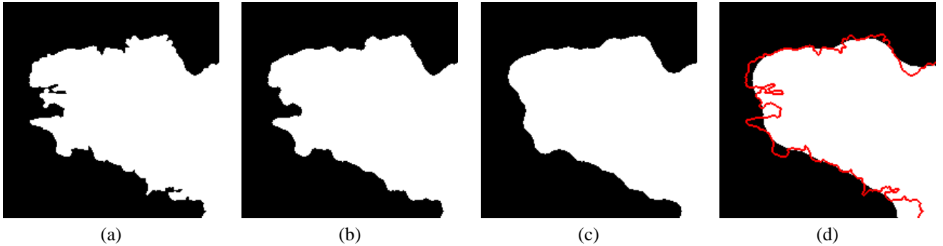
Figure 1. (a): a set X ; (b): ASF_3(X) ; (c): ASF_9(X) ; (d): the contour of X , superimposed to ASF_{25}(X) .
