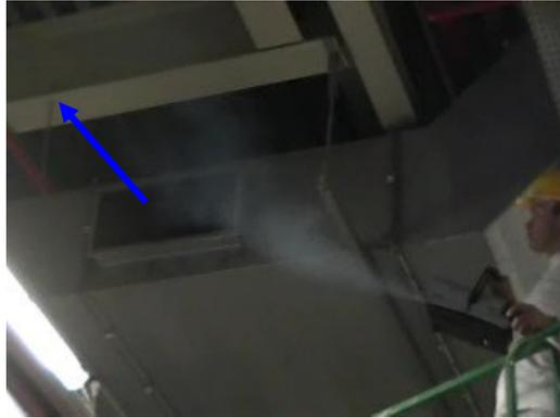
Figure 6 - Smoke injection at duct level.
