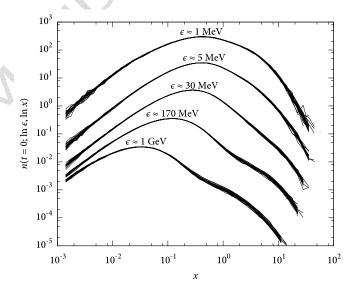
Fig. 9. Electron distributions  $n(t = 0; \ln \epsilon, \ln x)$  for different electron energies as a function of distance to the shower axis for 20 individual showers initiated by  $10^{18}$  eV protons. The curve set for 1 GeV is at the actual level; consecutive sets are shifted up by a factor of 10.
