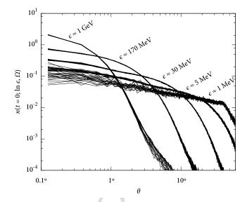
Fig. 3. Electron distributions  $n(t=0; \ln \epsilon, \Omega)$  at different electron energies as a function of momentum angle to the shower axis for 20 individual showers initiated by  $10^{18}$  eV protons.  $0^{\circ}$  is along the primary's trajectory,  $90^{\circ}$  is perpendicular to the shower axis.
