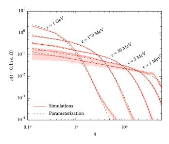
Fig. 5. Normalised average electron distributions  $n(t=0;\ln\epsilon,\Omega)$  (solid) for 20 proton showers at  $10^{18}$  eV with  $3\sigma$  statistical error margins (filled area). For each energy, corresponding parameterizations according to (8) are also drawn (dashed).
