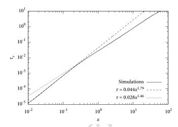
Fig. 22. Maximum density  $\tau_c$  as a function of lateral distance x at the shower maximum. Also shown are curves for  $x < x_0$  (dashed) and  $x > x_0$  (dotted) according to the parameterization in (21).
