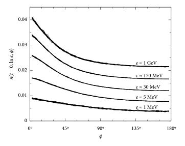
Fig. 7. Normalised simulated horizontal angular electron distributions for 20 individual showers initiated by  $10^{18}$  eV protons at different energies. Consecutive curve sets are shifted up by 0.005 to distinguish them better; curves for 1 MeV are at the actual level.
