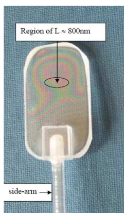
Figure 1: Photography of the NTC. Since NTC gap thickness is of order of visible light wavelength, interferometric pattern occurs. Region of L = \lambda = 800 nm is indicated, NTC has a sapphire side-arm.
