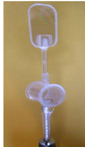
Fig.2 Photography of the multi-region cell. The nano-cell is seen in the upper part, while \sim 1 cm-long sapphire cell is shown in the middle part. MRC is fixed inside the oven with the help of the aluminum tube-holder which is tied to the side arm (only the top is seen at the bottom of the photo).
