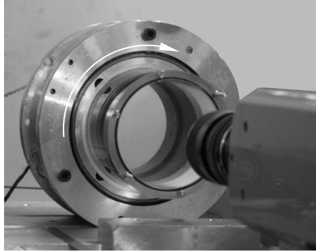
FIGURE 2. Photograph of the experimental device showing the tank (Rastello et al. 2009). In front of it is a high-speed camera. In the back the toothed belt can be seen.
