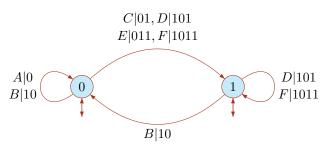
Fig. 1.35.: A 2-state encoder reflecting the legal concatenations.
