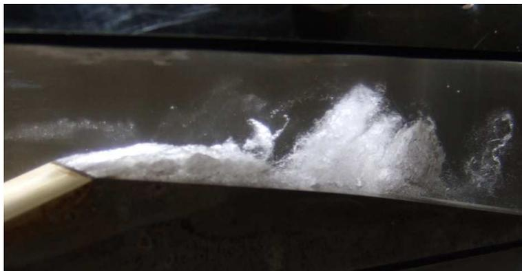
Figure 21: Photograph of the cavity, 8° Venturi.
