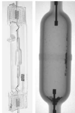
Figure 10. Hg-free lamp with outer envelope (left) and a X-ray (right) of the burner with spherical end-shapes.
