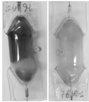
Figure 3.a Picture of one MS 400/BU/PS arc tube aged on CWA (12,500 hours, left hand picture) and one on VHF (10,000 hours, right hand picture).
