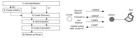
Fig. 2. Intra-cluster Routing Algorithm
