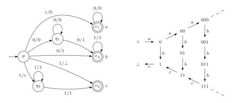
The path  $p \xrightarrow{0/0} q_1 \xrightarrow{0/1} r_2 \xrightarrow{1/1} r_2$  accepts the couple (001,011), the final state  $r_2$  is labelled by b thus there is a arc 001  $\xrightarrow{b}$  011 in the graph.
