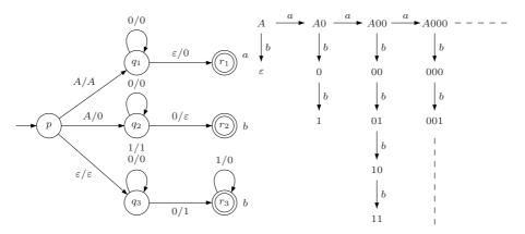
The encoding of the vertices of this tree relies on the fact that there are  $2^n$  *n*-tuples over  $\{0, 1\}$ . The transducer performs the binary addition.
