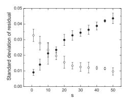
FIG. 3. Mean-square value of residuals of a Lorentzian (open circles) and Gaussian function (solid circles) fitted to the momentum distribution mapped through TOF.
