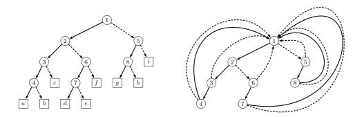
Fig. 3. A non synchronized Huffman code X on the left and its decoder on the right. The automaton on the right is not synchronized. Indeed, for any word w, the set of states reachable by w is either  $\{1,3\}, \{2,4\}, \{1,5\}, \text{ or } \{1,6\}.$
