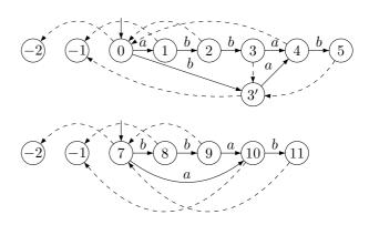
Fig. 7. Deterministic automata  $\mathcal{A}_0$  and  $\mathcal{A}_1$  accepting  $\operatorname{Fact}^{(0)}(y)$  and  $\operatorname{Fact}^{(1)}(y)$  respectively, with the period T=2 and y=abbab. The suffix links are represented by dashed edges.
