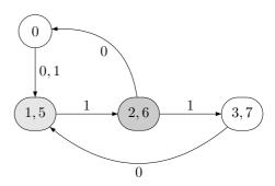
Fig. 6. The Shannon cover of  $S_{U,T}^{\sigma}$  for  $S={\rm MTR}(3),\,T=3,\,U=\{1\}.$  It is the minimal presentation of that of Figure 5.
