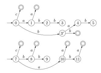
Fig. 8. Output tries  $\mathcal{T}_0$  and  $\mathcal{T}_1$  of Algorithm PERIODIC-MF-TRIES for the input tries  $\mathcal{A}_0$  and  $\mathcal{A}_1$  described in Figure 7. The sink states are double circled. The tries  $\mathcal{T}_0$  and  $\mathcal{T}_1$  accept  $\mathcal{MF}^{(0)}(y) = \{c, aa, bb\}$  and  $\mathcal{MF}^{(1)}(y) = \{c, ba, aa, aba\}$  respectively.
