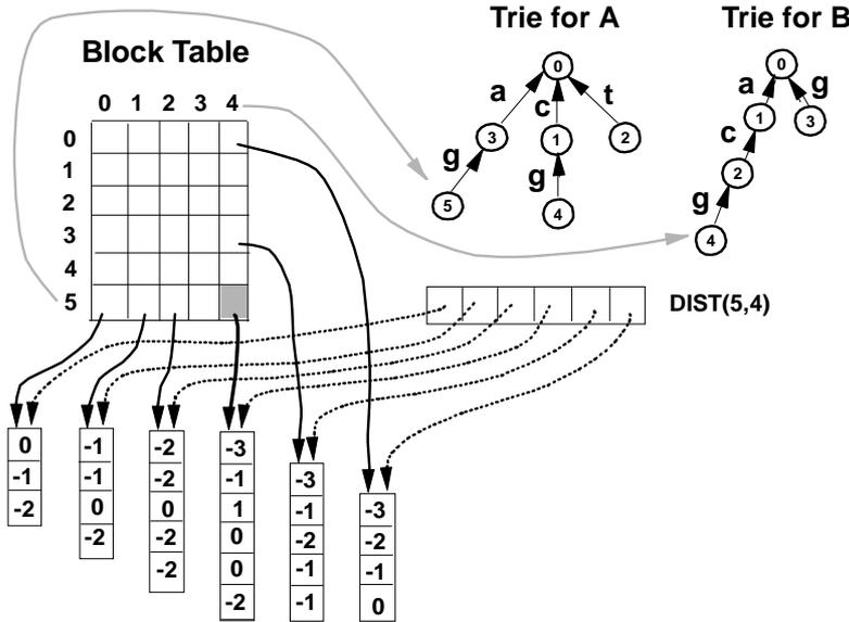
Figure 4: A table containing an entry for each block of the alignment graph. Entry  $(i, j)$  of the table represents the block which corresponds to node  $i$  in the trie for  $A$  and node  $j$  in the trie for  $B$ . The entry for each block in the table points to the start of its new  $DIST$  column. Also shown is the vector which contains pointers to all columns of the  $DIST$  for block  $(5, 4)$ , as obtained from its ancestor prefix blocks. This figure continues Figures 1, 2 and 3.
