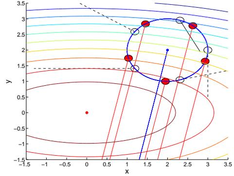
Fig. 6. Simulation of the distributed algorithm (12) by a circular formation of five agents centered at  $c = (2, 2)^T$ . The function  $\rho$  representing the source centered at the origin has elliptical level sets.
