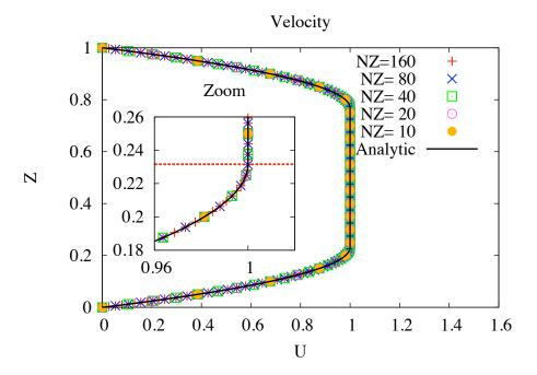
(a) Comparison of the longitudinal velocity profiles obtained by numerical simulations (symbols) for various meshes with the analytical solution (lines).
