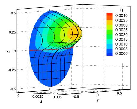
Figure 13: Velocity profile obtained by numerical simulations with the mixed-fluid model for the circular cross-section duct (6x896).
