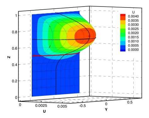
$Figure\ 10:\ Velocity\ profile\ obtained\ by\ numerical\ simulations\ with\ the\ mixed-fluid\ model\ for\ the\ square\ cross-section\ duct\ (6x20x40).$
