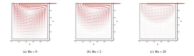
Figure 5: Velocity vector fields - Bingham varying from 0 to 20
