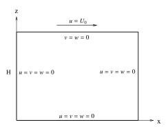
Figure 4: Sketch of the lid-driven cavity.
