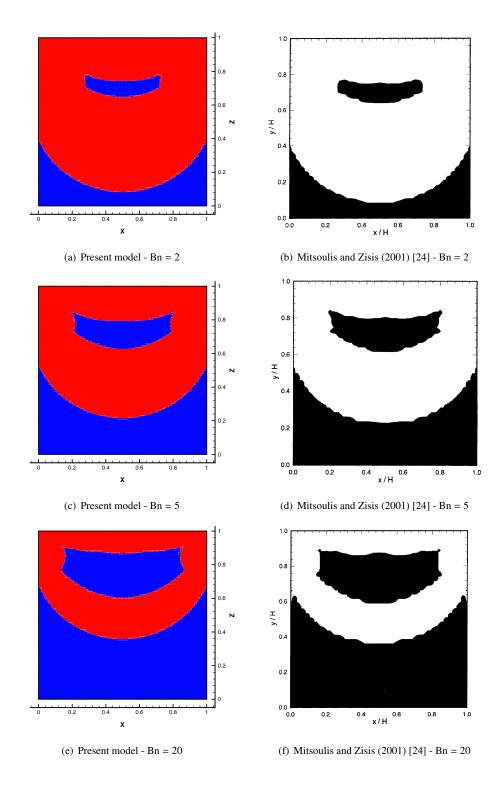
Figure 6: Comparison of the present numerical model results with those from Mitsoulis and Zisis (2001) [24] for the yield zone position in the lid-driven cavity for various Bingham number (Bn = 2, 5 and 20).
