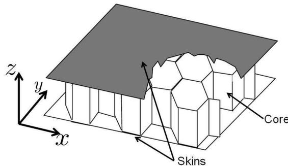
Figure 1: Geometry of the sandwich plate.
