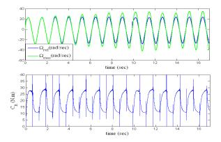
Fig. 12. Resistive torque  $(C_R)$  and rotation velocity tracking with applying MPPT algorithm when wind speed V is changed from 9m/sec to 10m/sec.
