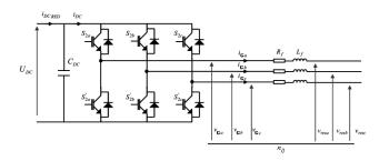
Fig. 6. Electric representation of the Grid-side converter.  $R_f, L_f$  are filtering components.
