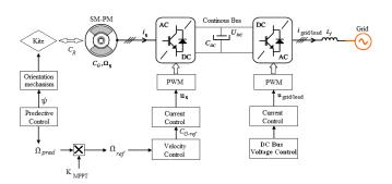
Fig. 7. General control scheme of the KGS.
