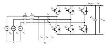
Fig. 5. Electric representation of the SM-PM-side converter. SM-PM is presented by Behn-Eschenburg model.  $C_{dc}$  is DC-bus filtering capacitor.
