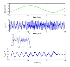
Fig. 13. Rotation Velocity ( $\Omega_G$ ), MS-PM phase current ( $I_{aG}$ ) and DC bus voltage ( $U_{DC}$ )
