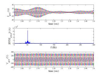
Fig. 14. Grid currents  $(I_{a,b,c})$ , phase current's frequential analysis  $(|FTT(I_a)|)$ , and Grid voltages  $(V_{a,b,c})$ .
