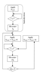
Fig. 8. Maximum Power Point Tracking (MPPT) algorithm.
