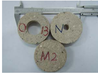
(b) Tubular SHPB specimen
