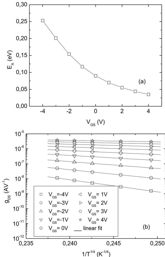
FIG. 1. Polycrystalline silicon TFTs are biased from weak to strong inversion ( $-4 \text{ V} \leq V_{GS} \leq 4 \text{ V}$ ). (a) Plots of the measured channel conductance activation energy as a function of the gate voltage. (b) Polycrystalline silicon TFTs channel conductance as a function of  $T^{1/4}$ .
