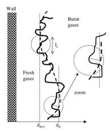
**Fig. 2.** The mean contour (bold dashed-line) is determined by filtering the scales larger than integral scale responsible of cyclic fluctuations. In each point of the instantaneous front, local roughness is measured in a disk of scale l<sub>i</sub> around the point. The wall-distance is measured from the point belonging to the mean contour, and obtained by drawing the perpendicular to the mean front to the wall.
