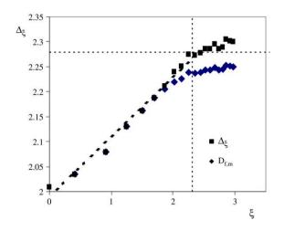
**Fig. 7.** Mean dimension  $D_{f,m}(d_d)$  over  $[l_p; d_d]$  and local fractal dimension  $\Delta_{\xi}$  as a function of scale logarithm  $\xi$  (with  $D_{f,m}(d_d) = [(\Delta[l_p] + \Delta_{\xi})/2]$ . Vertical dashed line indicates the integral scale. The linear fit (for wall distances belonging to  $[l_c; l_0]$ ) gives  $\Delta_{\xi} = 0.12 + 1.99\xi$ . The horizontal dashed line indicates the value  $\Delta_F^* = 2.28$  derived by using Ref. [14].
