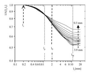
**Fig. 5.** Evolution of  $ln(1/\Lambda[l_c; l_i])$  as a function of x for wall-distances varying from 0.3 mm  $\leq d_d \leq 3.8$  mm. The arrow on the right indicates decreasing values of wall-distance from 3.9 mm to 0.3 mm. Vertical dashed-lines indicates the inner cut-off scale  $l_c$ , the scale  $l_p$  used for the measurement of  $\Delta_{\xi}$ , the integral scale  $l_0$  and the outer cut-off scale  $l_M$ .
