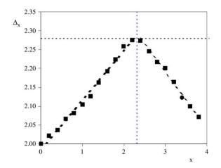
**Fig. 6.** Local fractal dimension  $\Delta_x$  as a function of scale logarithm x. The linear fit corresponding to the first zone  $[l_c; l_0]$  leads to  $\Delta_x = 0.13x + 1.99$ . The linear fit in the symmetrical zone gives  $\Delta_x = 0.15x + 2.63$ . Vertical dashed line indicates the integral scale. The horizontal dashed line indicates the value  $\Delta_F^* = 2.28$  derived by using Ref. [14].
