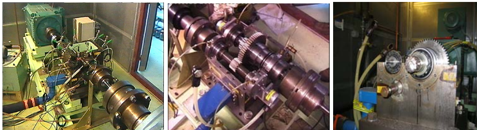
Fig.1: Left: gear testing device, middle: tested gears, right: cracked gear coupling. The gear coupling that links the training motor shaft to the gear shaft appears in the lower right corner of the middle figure.
