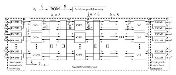
Fig. 6: Stochastic cortex decoder made up of a ROM, a serial-to-parallel memory and a fully parallel multiple stream stochastic core.
