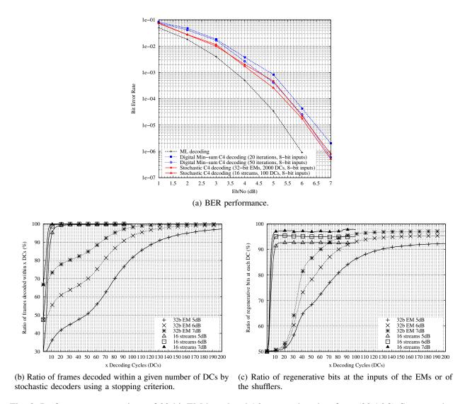
Fig. 8: Performance comparison of 32-bit EM-based and 16-stream decoders for a (32,16,8) Cortex code.
