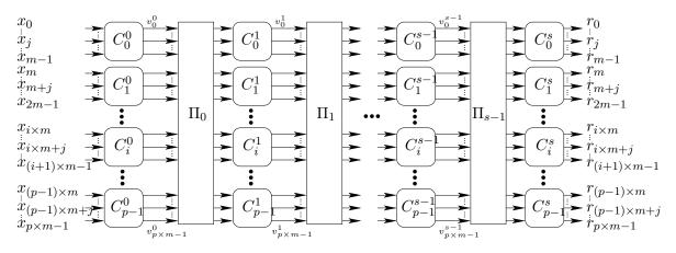
Fig. 1: Cortex encoder made up of s interleaving stages and  $(s+1) \times m$  component encoders.
