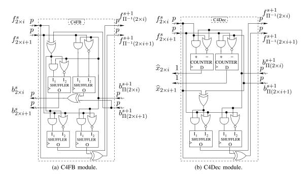
Fig. 7: Stochastic multiple stream processing modules computing forward/backward messages and decisions. All the shuffler inputs V, which give the shifting value and are driven by the same signal, are not mentioned.
