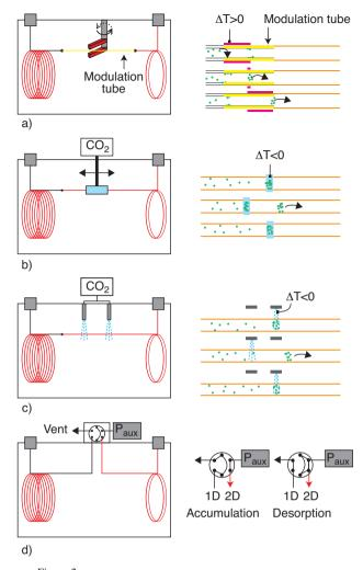
Figure 2 The different modulation systems and their process of modulation. From top to bottom : Sweeper modulator - Longitudinally Modulation system - Dual-jets  ${\rm CO_2}$  modulator - Valve-based modulator.
