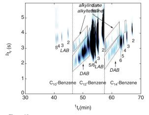
Figure 10 GC×GC chromatograms of the product from linear alkylbenzene (LAB) synthesis. The number refers to the position of the benzyl group on the main alkyl chain.
