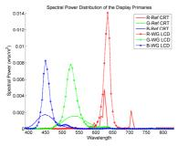
Fig. 3. Spectral Power Distribution of the CRT and the LCD used in the experiments
