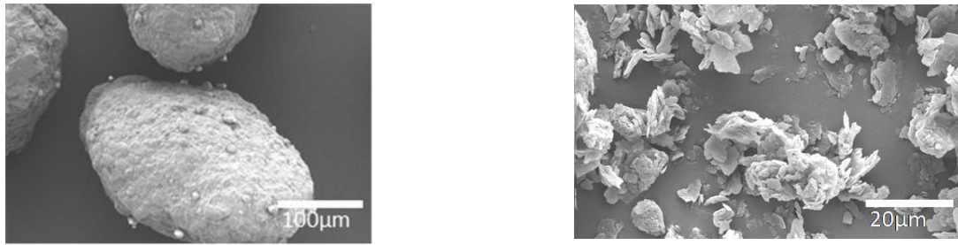
Figure 1. SEM images of Suglets(a) and MgSt(b).
