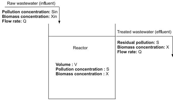
Figure 1: Simple example of a bioreactor. The reactor volume is often calculated such that the residual pollution concentration is lower than a limit value  $S_{lim}$
