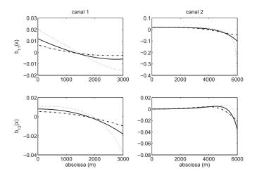
FIGURE 19. Functions  $b_{11}(x)$  and  $b_{12}(x)$  of the distributed modal decomposition for canals 1 and 2 in accelerating  $(\cdots)$ , uniform (-) and decelerating (-,-) flow.
