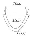
FIGURE 1. Section of an open channel. Definition of the wetted perimeter P, wetted area A and top width T.
