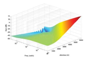
FIGURE 8. Spatial Bode plots of transfer function  $g_{11}(x,s)$  for canal 2
