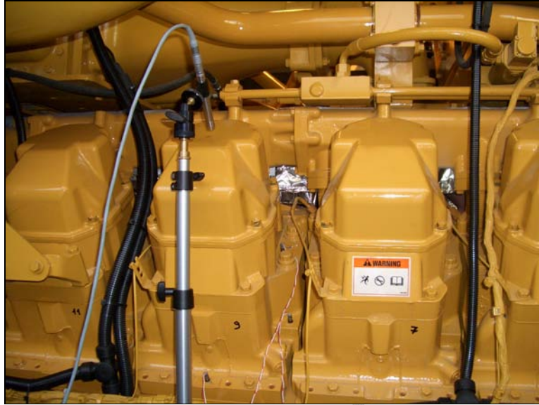
Figure 4 – Vibration and acoustic signal acquisition on the cylinder n. 9 of the CAT G3516B engine
