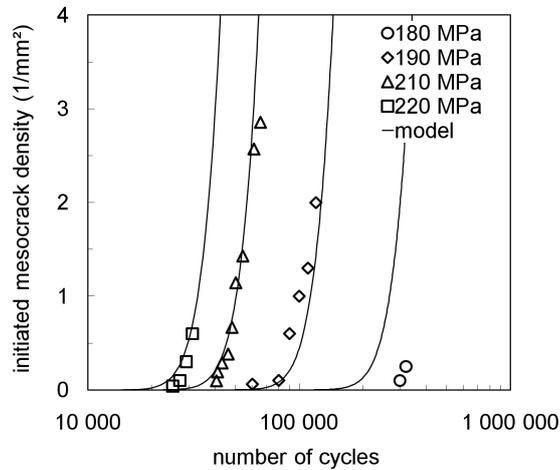
Figure 10: comparison between experimental crack densities evolution and model prediction
