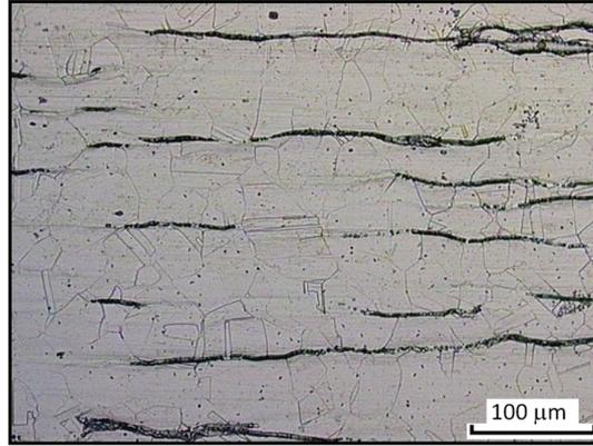
Figure 1: 304L microstructure made of austenitic grains (gray) with ferritic residual grains (black).
