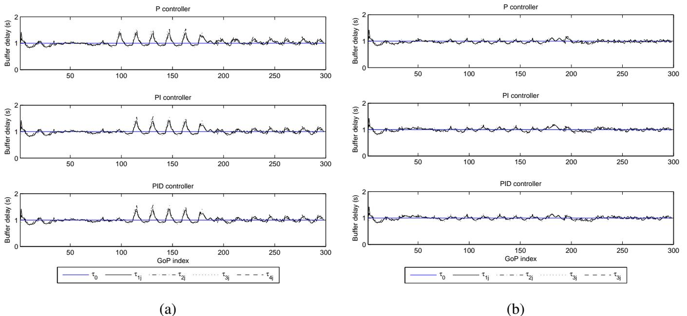
Figure 9. Buffering delay evolution of the 4 multiplexed programs using P, PI, and PID controller with  $W = 2$  (a) and  $W = 4$  (b) in the encoder control process with constant channel rate
