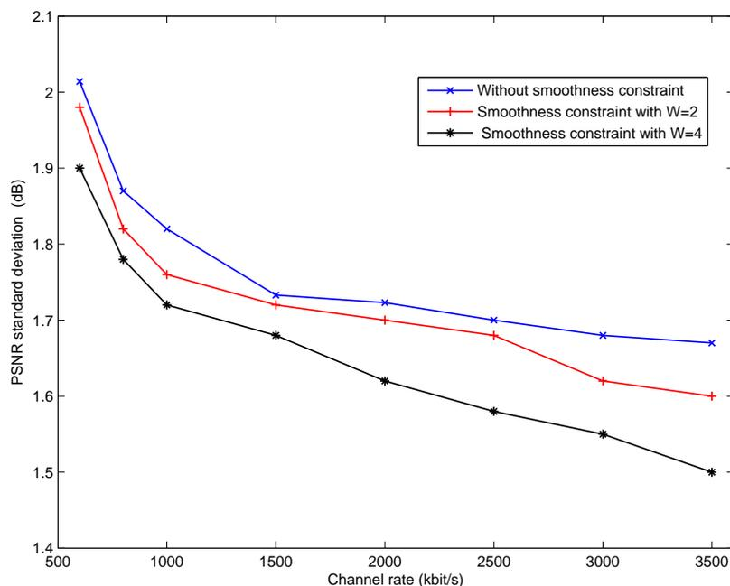
Figure 7. Standard deviation of the PSNR without smoothness constraint, with smoothness constraint when  $W = 2$  and  $W = 4$  for different channel rates
