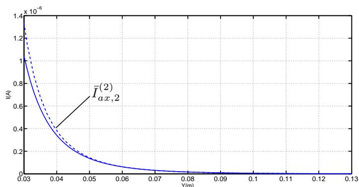
(b) Current of  $I_{ax}$  in function of  $Y$  measured by the electrode  $\mathcal{E}_2$ FIGURE 10 – Currents measured by the electrodes  $\mathcal{E}_2$ , (solid lines : model, dotted lines : BEM).
