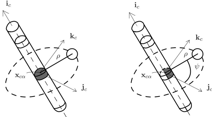
FIGURE 14 – The role played by the components  $I_{ax}$  (left) and  $I_{lat}$  (right) for electrolocation.  $I_{ax}$  is the stronger component of the current perturbation, and gives information on the height along direction  $\mathbf{i}_c$  and the distance  $\rho$  from the sensor axis at which we can locate the object while  $I_{lat}$  disambiguates the azimuth angle  $\psi$ .
