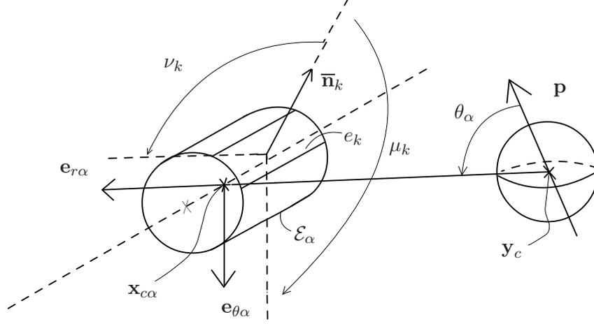
FIGURE 6 – The perturbation  $I^{(1)}$ . A schematic view of one perturbed  $\mathcal{E}_\alpha$  of the sensor is depicted. The perturbation  $I^{(1)}$  gives lateral information by measuring the net flux of  $\gamma\mathbf{E}_1$  across the electrodes  $e_i$ . Like the fish, the sensor is able to know which "side" of its body is more affected by the presence of the object.
