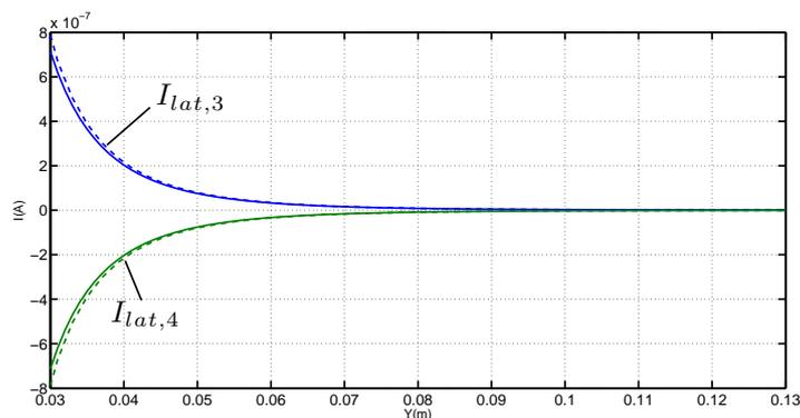
(a) Currents of  $I_{lat}$  in function of  $Y$  measured by the electrodes  $e_{i=3,4}$ .
