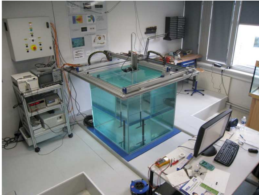
FIGURE 11 – The experimental set-up. The cartesian robot permits a movement in an horizontal plane with a precision equal to 0.1 mm.
