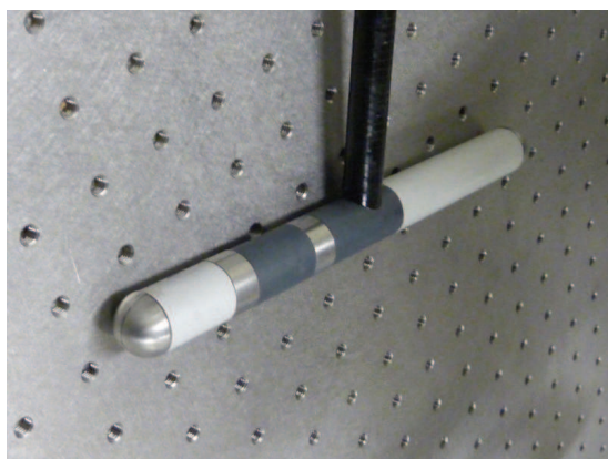
FIGURE 3 – (top) Picture of a 7-electrode slender sensor organized in 4 polarizable rings, 3 of them being divided in two half rings allowing two lateral (left and right) measurements. (bottom) General schematic view of the slender sensor with its parametrisation.
