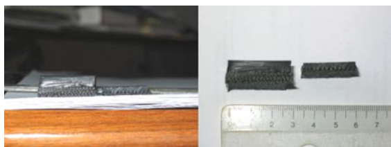
Fig. 20 Pictures of tyre sections: Lab 1 ( thick tyre on the left side of both pictures ) and Lab 2 ( thin tyre on the right side of both pictures )
