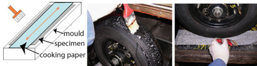
Fig. 5 Anti-sticking procedure. It consists of placing a sulfurized paper on the top surface of the specimen and spreading a greasy soap on it and on the tyre
